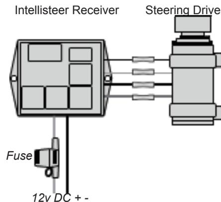
**NOTE:** For a standalone drive installation the four Course Computer wires (Yellow, Yellow/Green, Brown and Pink) are not used, and should be wrapped with electrical tape and secured.
